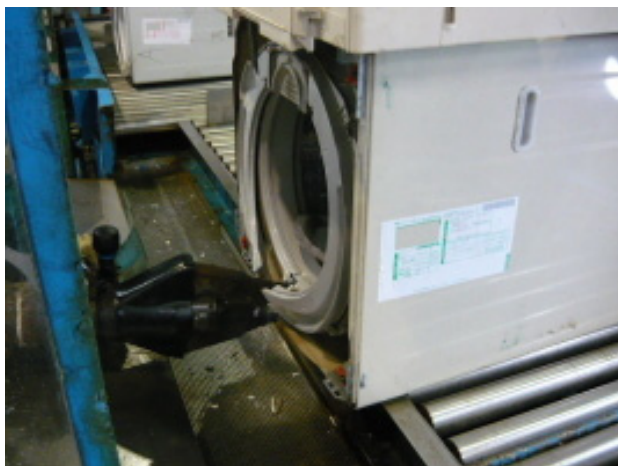
To keep shredding machines and recycled metals from rusting, salt water in the ring element at the top of the washing tank is taken out by cutting machines.
