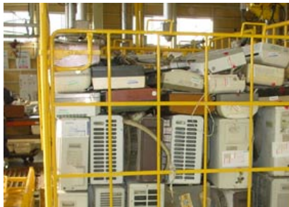
At a carry-in entrance of a home appliance recycling plant: Indoor and outdoor units are loaded in cargo containers.
