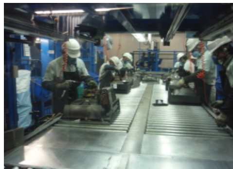
After back covers are removed, major components such as CRTs and printed circuit boards are manually removed.
