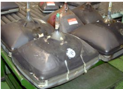
Removed CRTs: They are recycled as glass after separation, crushing and cleaning.
