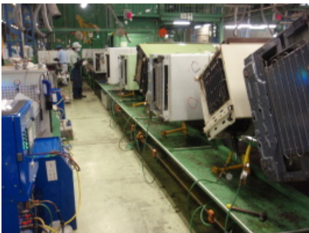
Refrigerant fluorocarbons are recovered by dedicated equipment. Recovered fluorocarbons will be destructed at designated treatment facilities.
