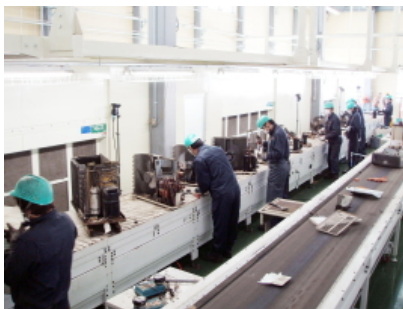
Major components of outdoor units such as printed circuit boards, compressors, and heat exchangers are manually removed after recovering refrigerant fluorocarbons.
