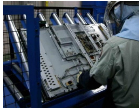
Large-sized LCD TVs are effectively dismantled on a designated workbench.
