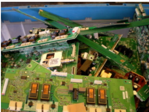
Printed circuit boards removed from LCD TVs: They will be recycled at designated treatment facilities.
