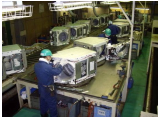
After removing motors and printed circuit boards, top covers are removed.
