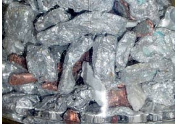
Recovered mixture of metals: They are included aluminum and copper.
