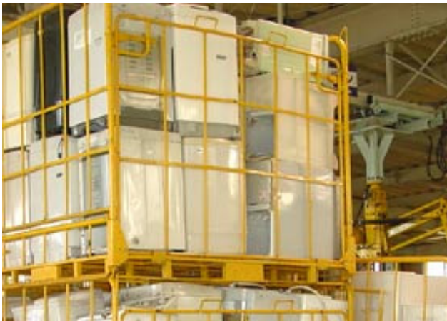
At a carry-in entrance of a home appliance recycling plant: Washing machines are loaded in cargo containers.
