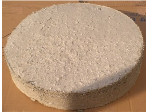
Recovered urethane: Urethane, utilized for heat insulation in refrigerators, is compacted after its pulverization. Fluorocarbons which are contained in heat insulation are recovered in a sealed shredder.
