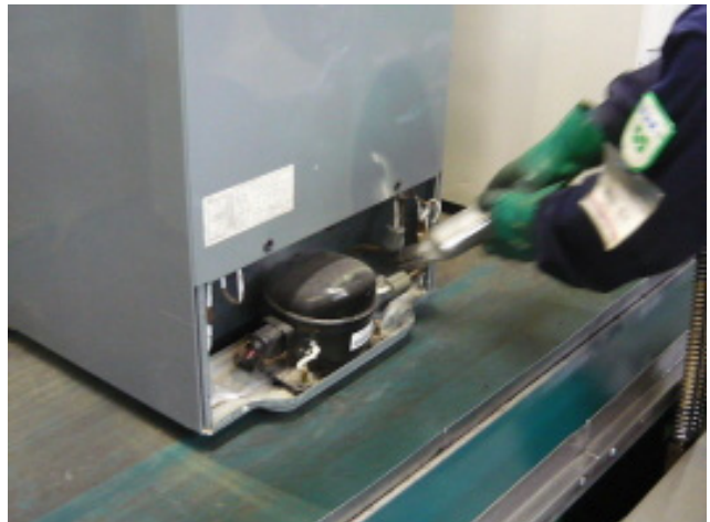
After recovering refrigerant fluorocarbons, compressors are removed by cutting pipes.
