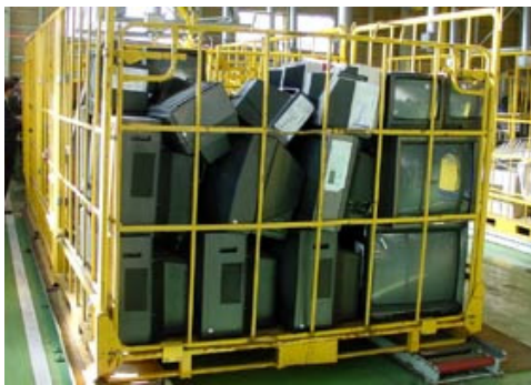
At a carry-in entrance of a home appliance recycling plant: Television sets are loaded in cargo containers so as not to break the cathode-ray tubes.
